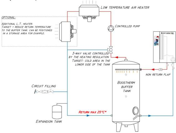
> Assembly for combined low temperature heating and DHW production
