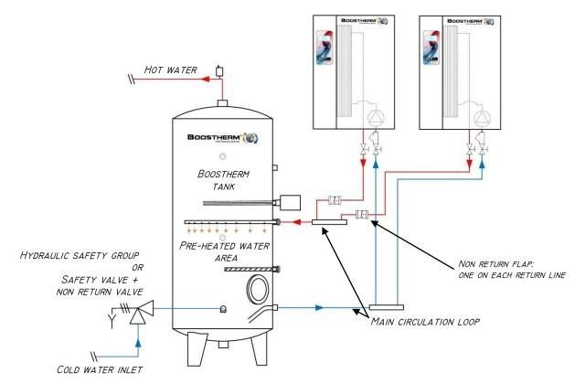
> Assembly with 2 buffer tanks in parallel.
